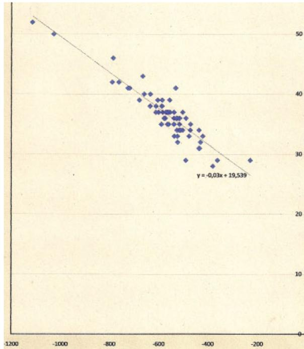
Fig. 3. Dependence of temperature on depth from the measurements of maximum temperature in mine forbores. Calculated values: Temperature gradient  $G_{100} = 3,0^{\circ}/100$  m. Correlation coef.  $-0,905$
