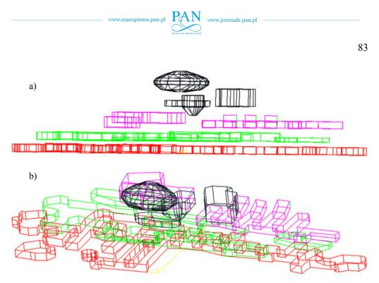
Fig. 4. Summary presentation of the spatial models of chambers in the vicinity of the Warszawa Chamber and Levels from II to III adopted for numerical modelling: a) view from the south on the chamber model, b) view "from the top" towards south-east (Cieślik et al., 2009)
