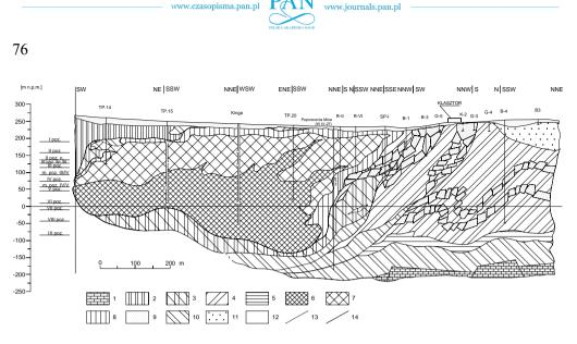
Fig. 2. Geological cross-section of the "Wieliczka" salt bed (Szybist, 2011)
