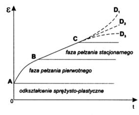
Fig. 3. Phases of rock salt strain (Ślizowski, 2006)
