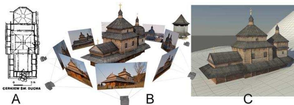
Fig. 1. Technical projection and photography scheme: A – technical projection of the church; B – scheme of photographing from the outside of current church; C – view of the church before 1736
