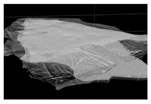
Fig. 4. Top and Bottom of lignite, drill holes and topography DTM (Haxhiu, 2004)
