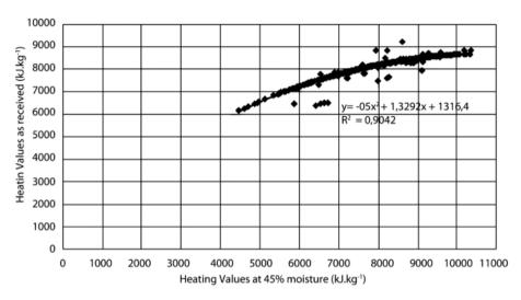
Fig. 1. Relation of heating values on 45 % moisture to as received basis (Haxhiu, 2004)
