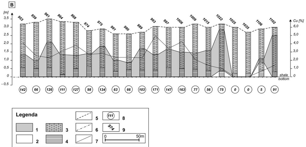
Fig. 4. Simplified cross-section of deposit series variability in division B: 1 – deposit series, 2 – barren rocks, 3 – dolomite, 4 – shale, 5 – gallery roof, 6 – gallery floor, 7 – Cu content in deposit series [%], 8 – Cu yield [kg/m<sup>2</sup>], 9 – sample number
