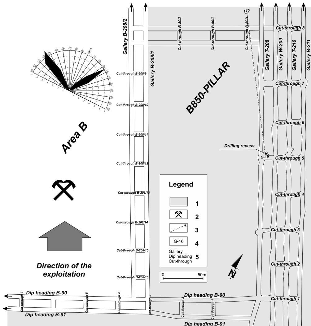
Fig. 1. Simplified configuration of development works applied in the Polkowice-Sieroszowice mine:
