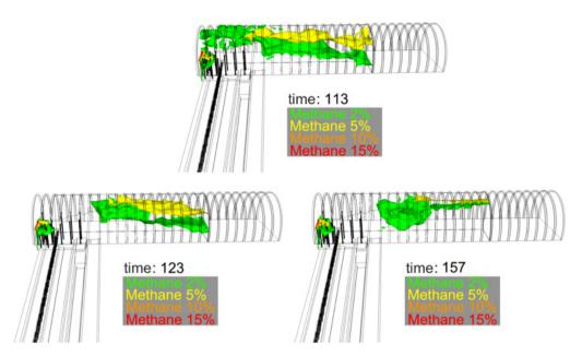
Fig. 8. Selected temporal instants in the process of ventilating the upper corner area
