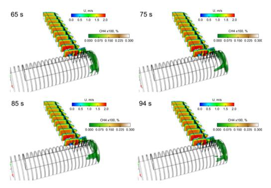
Fig. 4. Selected time instants of the air-methane mixture flow; the "steady state"
