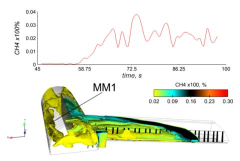
Fig. 7. The location and registration of a virtual methane meter – MM1
