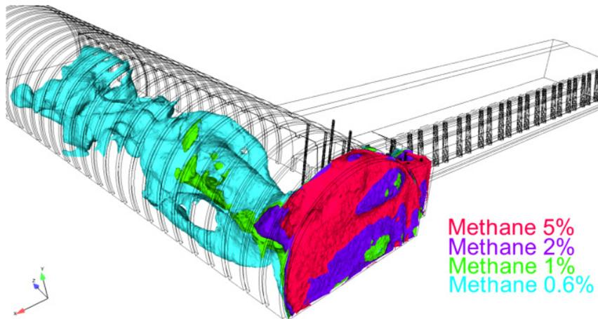
Fig. 5. The isosurfaces of the distribution of methane concentrations on the „cap”
