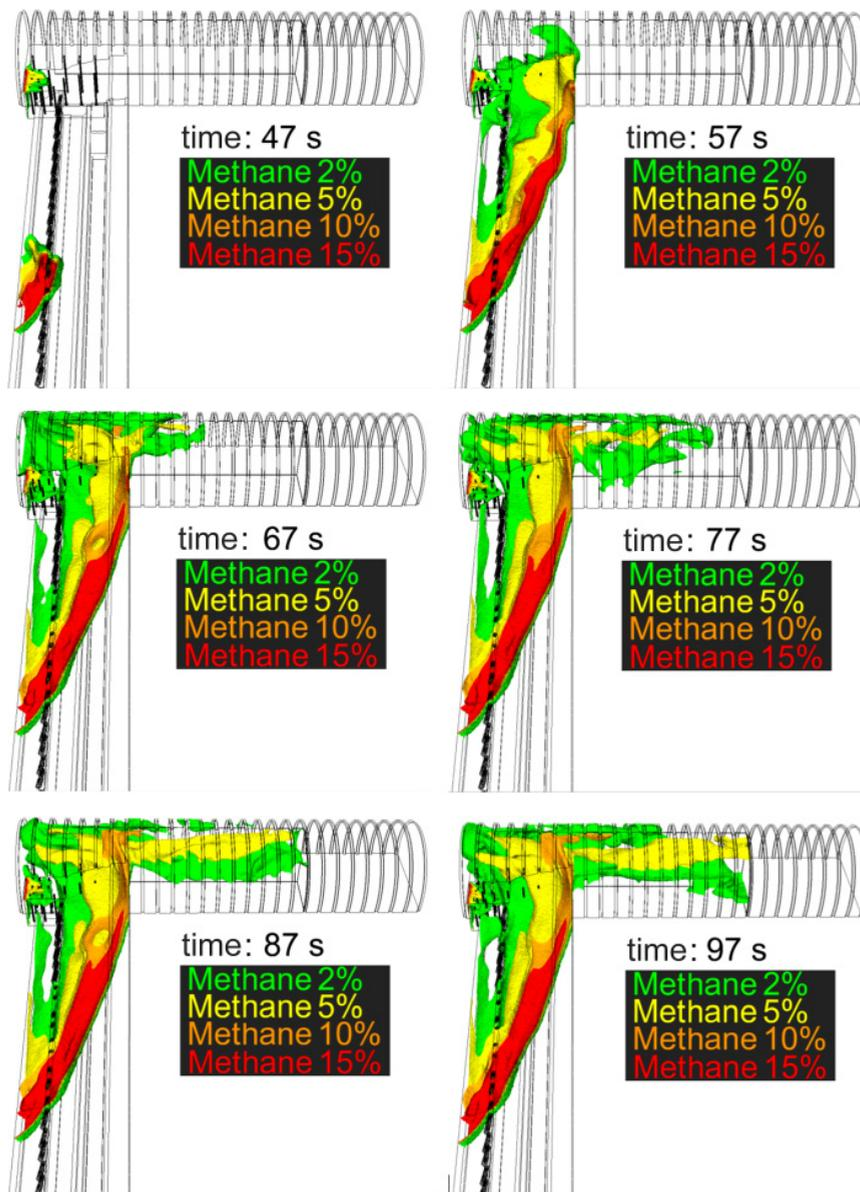
Fig. 6. Selected time instants of a sudden air-methane mixture outflow
