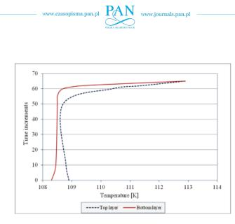
Fig. 5. Changes of temperature of liquefied natural gas containing nitrogen in a tank
