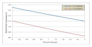
Fig. 8. Influence of nitrogen content on LNG bubble point
