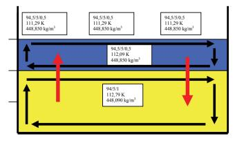
Fig. 4. LNG tank. Modeling of stratification. There is a rise in temperature in lower layer and consequently stratification of liquid in tank (*rollover*)
