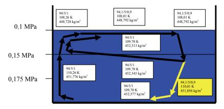
Fig. 1. LNG tank. Modelling of initiation of LNG with nitrogen stratification
