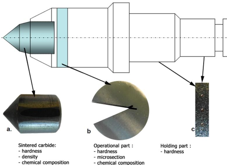
Fig. 10. Tangential-rotary pick with marked measurement points
