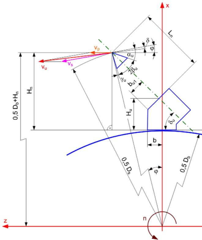
Fig. 2. Parameters of the holder and tangential-rotary pick fixing
