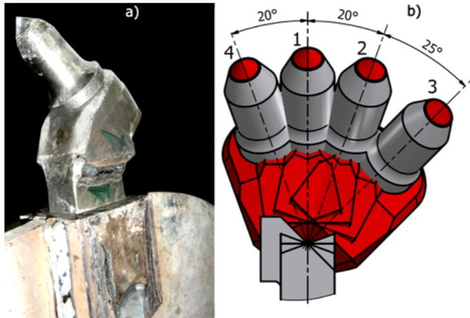
Fig. 14. Example of the pick system with numbered picks
