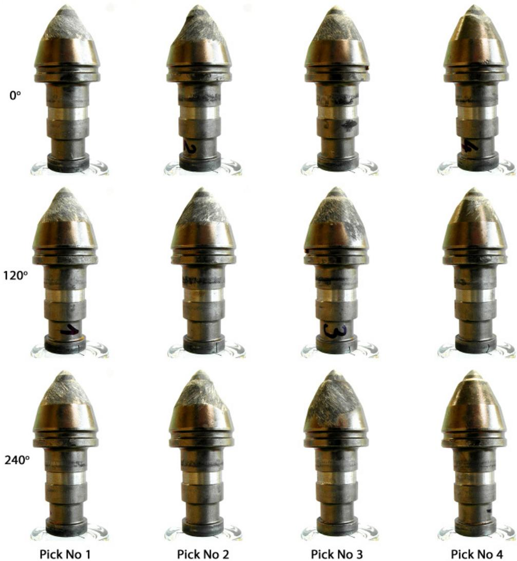
Fig. 15. Examples of tangential-rotary picks after examinations
