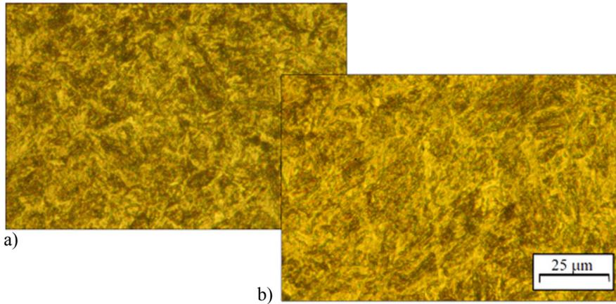
Fig. 11. Tempered martensite – ex ample structure of tested pick body material
