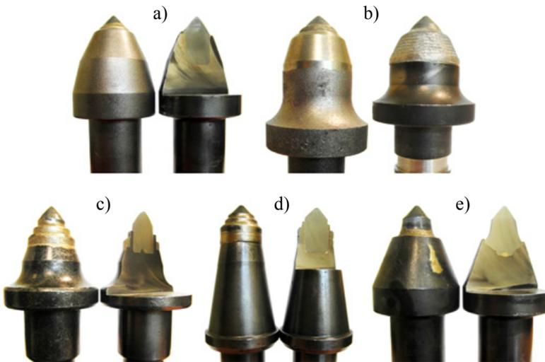
Fig. 6. Options of additional protection of the tangential-rotary picks against abrasive wear (Sandvik, 2013)
