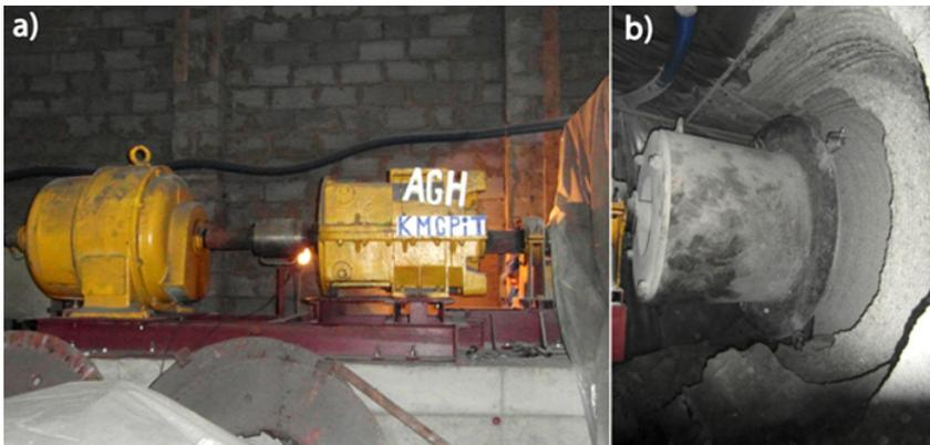
Fig. 13. Testing stand for examination of the quality of tangential-rotary picks
