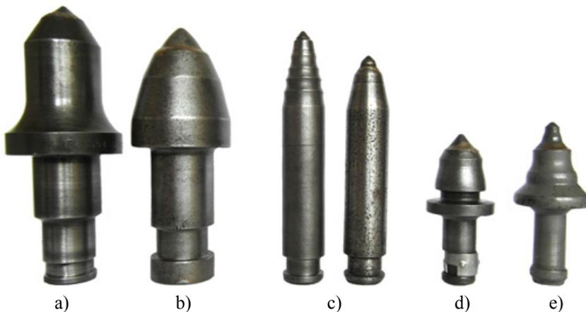
Fig. 5. Tangential-rotary picks used for: a) longwall shearers, b) roadheaders, c) shearers used for salt mining, d) milling machines for concrete cutting, e) milling machines for asphalt cutting
