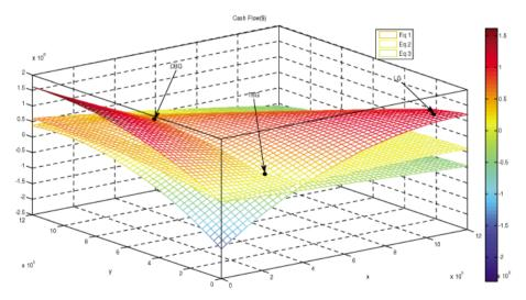
Fig. 2. The cash flow surface in light of governing limitations and limiting (LG), dual balancing (DBG) and triplet (TBG) cut-off grades are specified
