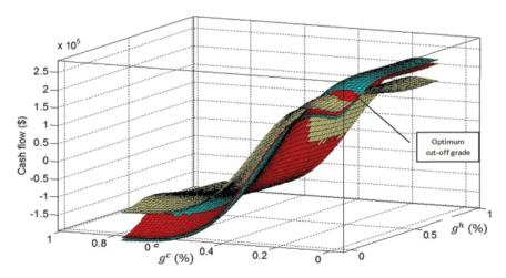
Fig. 4. The geometric location of optimum cut-off grade
