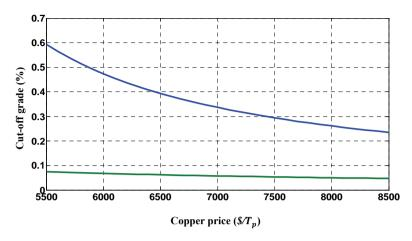
Fig. 6. The effect of copper price variations on optimum cut-off grades (mining capacity is the limiting factor), concentration cut-off grade (---), Heap leaching cut-off grade (---)
