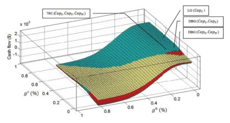
Fig. 3. The limiting, dual and triple balancing cut-off grades of the hypothetical mine
