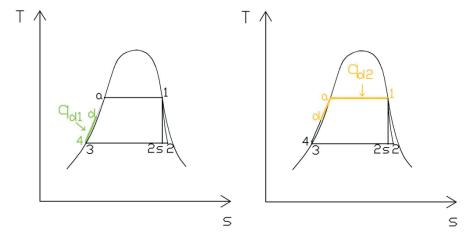
Figure 1. Heating of working fluid by the low temperature waste heat,  $\dot{Q}_{in 1}$ .
