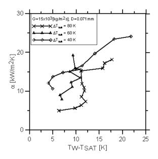
Figure 7. Nucleate boiling heat transfer coefficients of evaporating water jet for the nozzle diameter  $D=0.071~{\rm mm}.$
