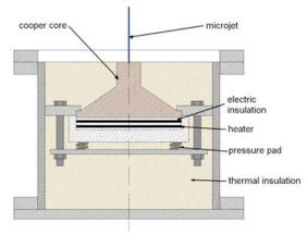
Figure 2. Cross-section of the probe.
