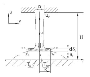
Figure 3. Scheme of rapidly evaporating microjet.
