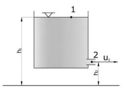
Figure 4. Outflow from the large tank through a small hole.
