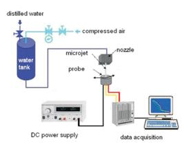
Figure 1. Schematic diagram of test section.
