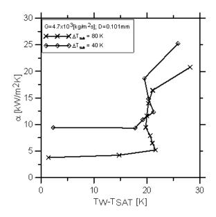
Figure 6. Nucleate boiling heat transfer coefficients of evaporating water jet for the nozzle diameter  $D=0.101~{\rm mm}.$
