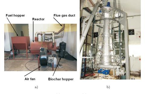
Figure 1. Examples of horizontal (a) and vertical (b) reactors for the thermal treatment of biomass fuels at the Czestochowa University of Technology.
