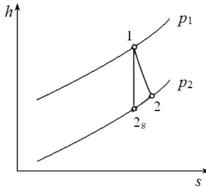
Figure 2. Isentropic expansion 1-2<sub>s</sub> in relation to the real expansion 1-2 from pressure  $p_1$  to  $p_2$ .
