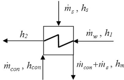
Figure 4. Schematic of the open-feedwater heat exchanger.
