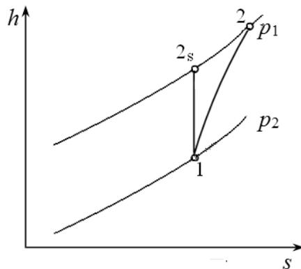
Figure 3. Isentropic pumping 1-2<sub>s</sub> and real pumping 1-2 from pressure  $p_1$  to  $p_2$ .
