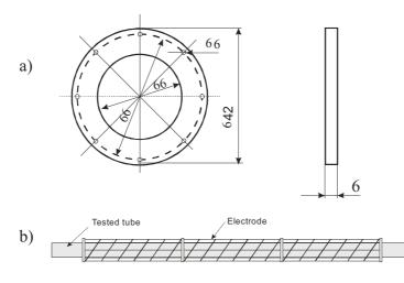
Figure 15: Geometry of a concentric electrode: a) polytetrafluorethylene (PTFE) distance rings; b) tube fitted with the electrode.
