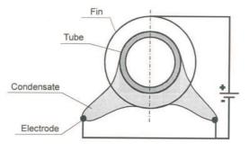
Figure 18: The idea of the EHD condensate drainage by means of the double electrode system.
