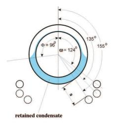
Figure 20: Geometry of the tube-double electrode systems. The angle  $\Phi$  denotes the flooding angle (corresponding to the tube circumference free of the retained condensate) for tube No. 6.
