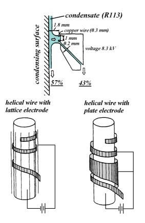
Figure 2: Condensation heat transfer enhancement on vertical tubes [12].
