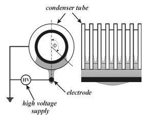
Figure 4: The idea of the condensation enhancement by EHD condensate drainage.
