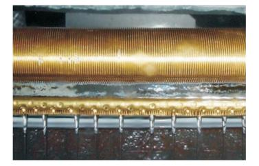
Figure 21: The condensate flow pattern between the tube and the electrode, tube No. 6,  $\omega = 135^{\rm o}.$
