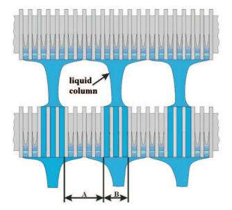
Figure 1: The condensate flow pattern according to Honda *et al.* [10]: A – unaffected region of vapor condensation, B – affected region by condensate inundation.
