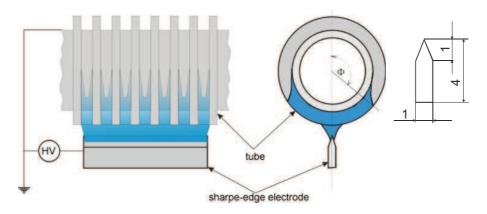
Figure 12: Electrohydrodynamic condensate drainage by means of a sharp-edge electrode: a) physical situation, b) geometry of the electrode given in mm.
