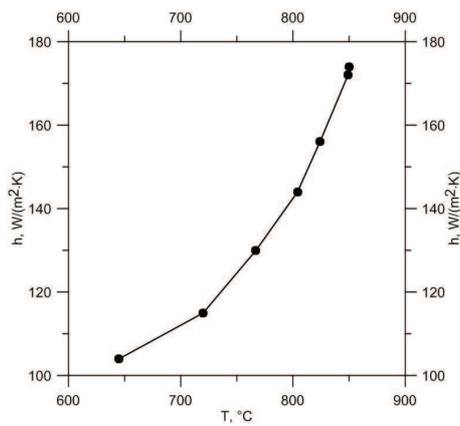
Figure 6. The heat transfer coefficient as a function of the flue gas temperature.
