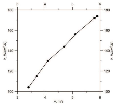
Figure 7. The heat transfer coefficient as a function of the flue gas velocity.
