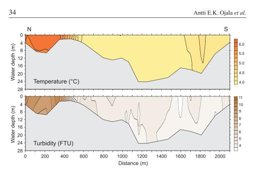
Fig. 4. The CTD profile data presented here for Revvatnet were collected along an approximately N-S-oriented survey line (20 points) in the middle of the lake. The upper panel indicates the 2D distribution of temperature and the lower panel the turbidity of the water column. The data were collected on June 17, 2013.
